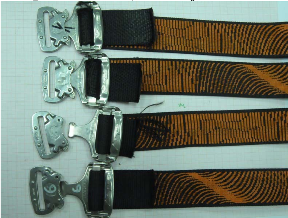
Test pieces after breaking load test
